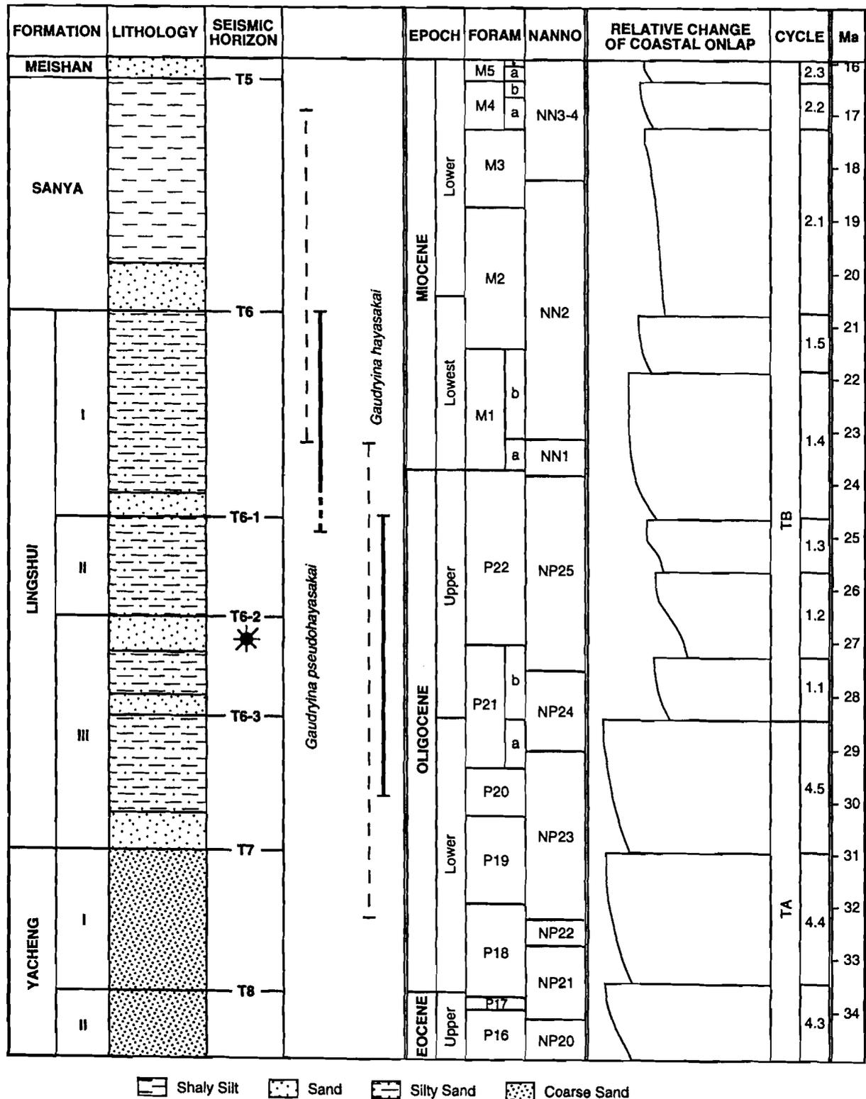
Figure 2. General stratigraphic section for the Lower Miocene to Upper Eocene of the Qiong Dong Nan Basin. Arrows mark the position of microfossil datums and their numerical ages in Ma. Chronostratigraphy is from Berggren *et al.* (1995) and the coastal onlap curve is from Haq *et al.* (1987, 1988) rescaled to the Berggren *et al.* (1995) chronostratigraphy. Dashed lines indicate ranges on Taiwan.
