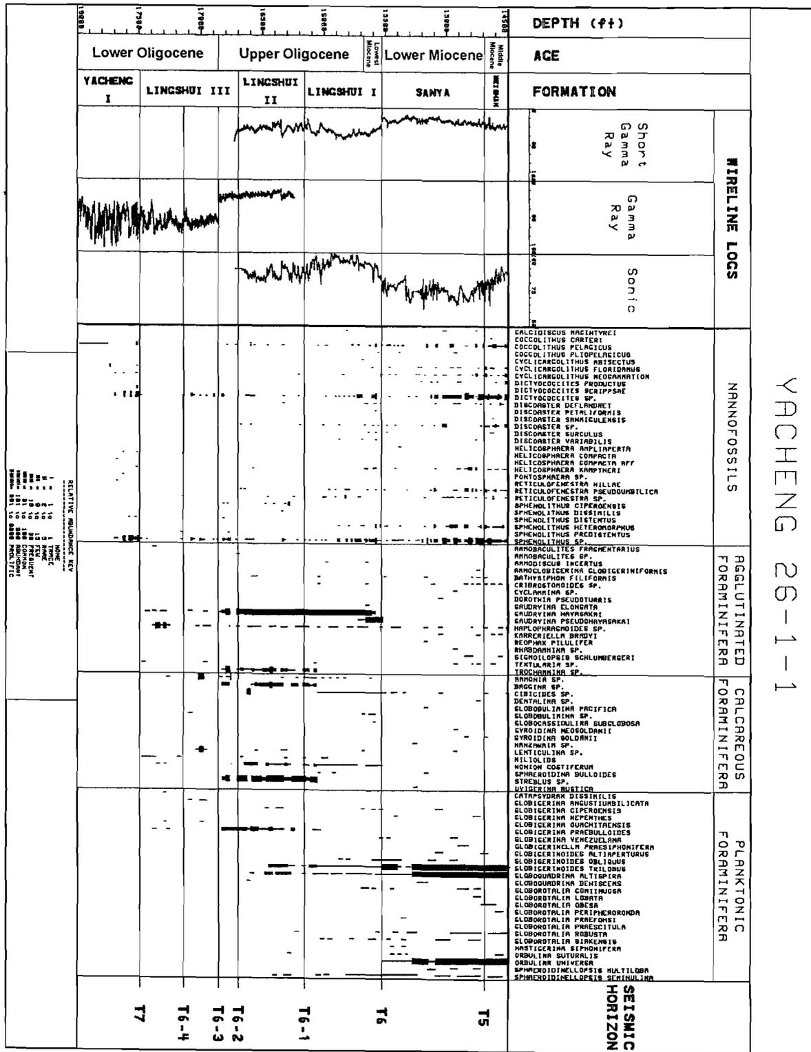
Figure 5. Microfossil distribution in Yacheng 26-1-1 well between 14,500' - 18,000' relative to wireline logs, and interpreted seismic horizons, formations, and ages.
